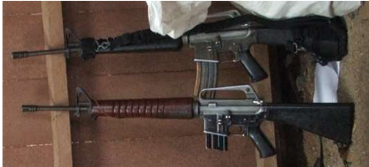
M16A1s: the top one has a 30-round magazine, while the bottom one has a, 20-round magazine and wooden handguard
