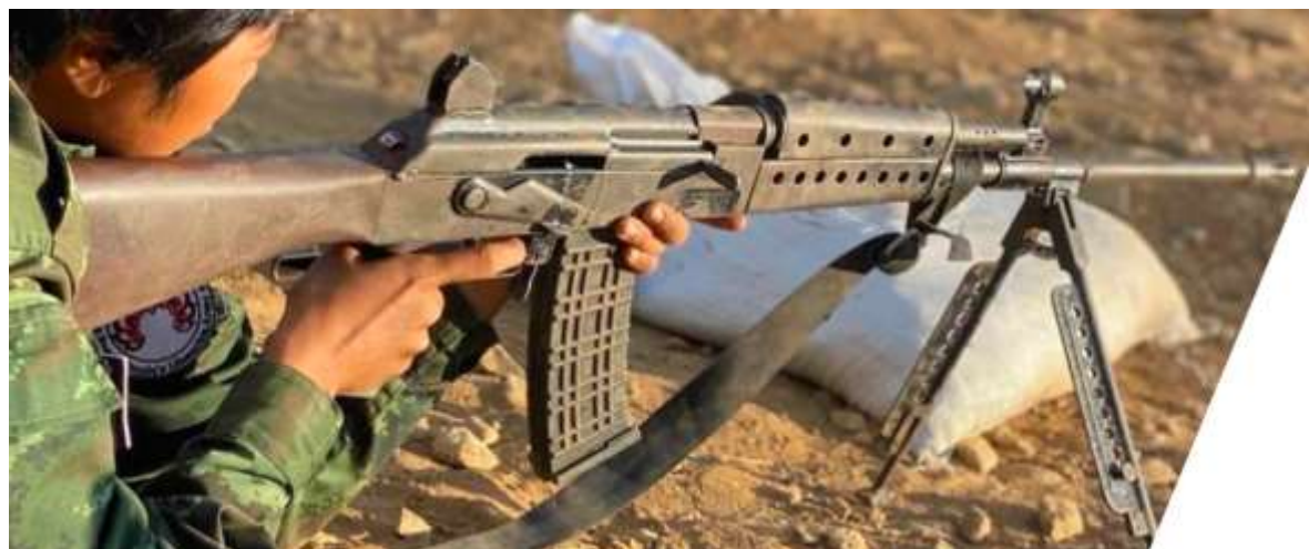
MA-2 Mk. II with polymer magazine and M-60-styled bipod mounted close to front sights
