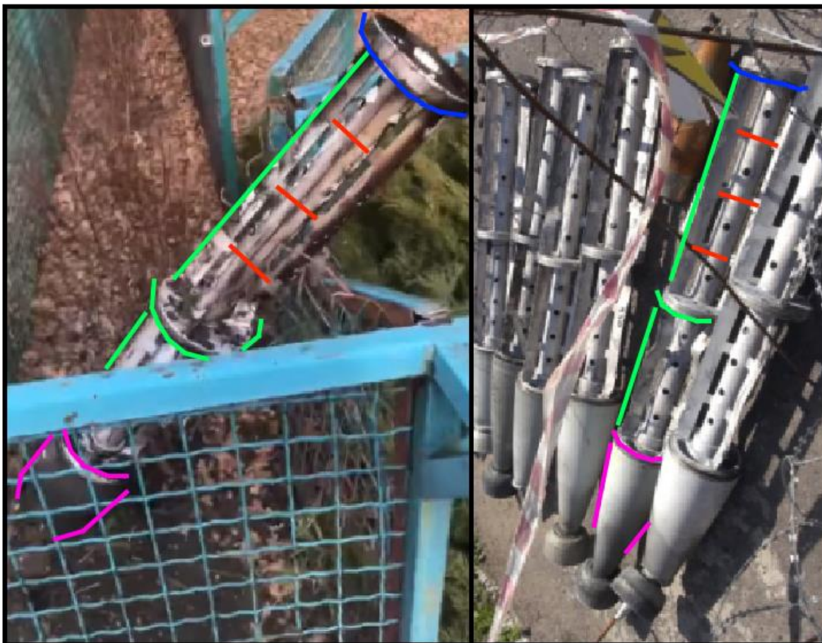
Figure 10: Comparison of the cargo rocket that landed at Feldman Ecopark (left) with the Uragan cluster munition rocket 9M27K series used in 2014 against Ukraine (right).
