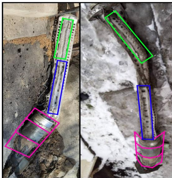
Figure 14: A comparison of the remains of the missile that landed on Mykolaiv Zoo on 23 March (left), and the missile remains identified as belonging to the Russian 9M54 series (right). 5960
