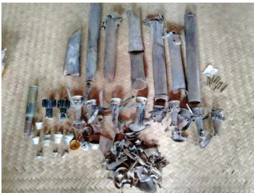
Figure 10: Aftermath of airstrike debris allegedly gathered from the 16 September 2022 airstrike attack in Let Yet Kone village, Sagaing State. Confirmed S-5 rocket remnants are shown. (Source omitted to maintain the safety of the social media user).
