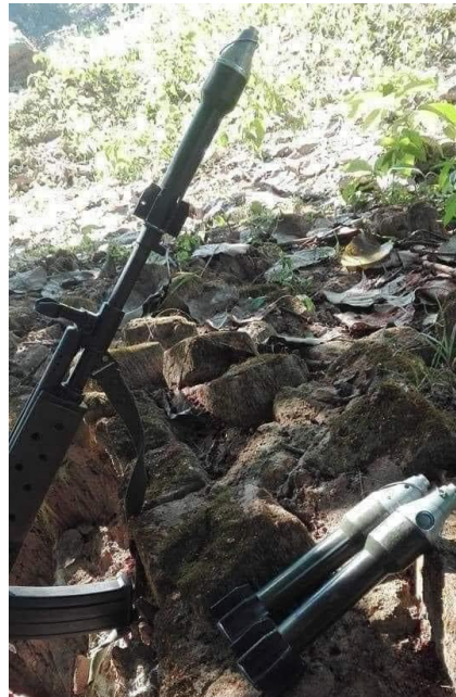
Image 43: MG-2 grenade attached to MA-1 Mk. I assault rifle, sourced from here .
