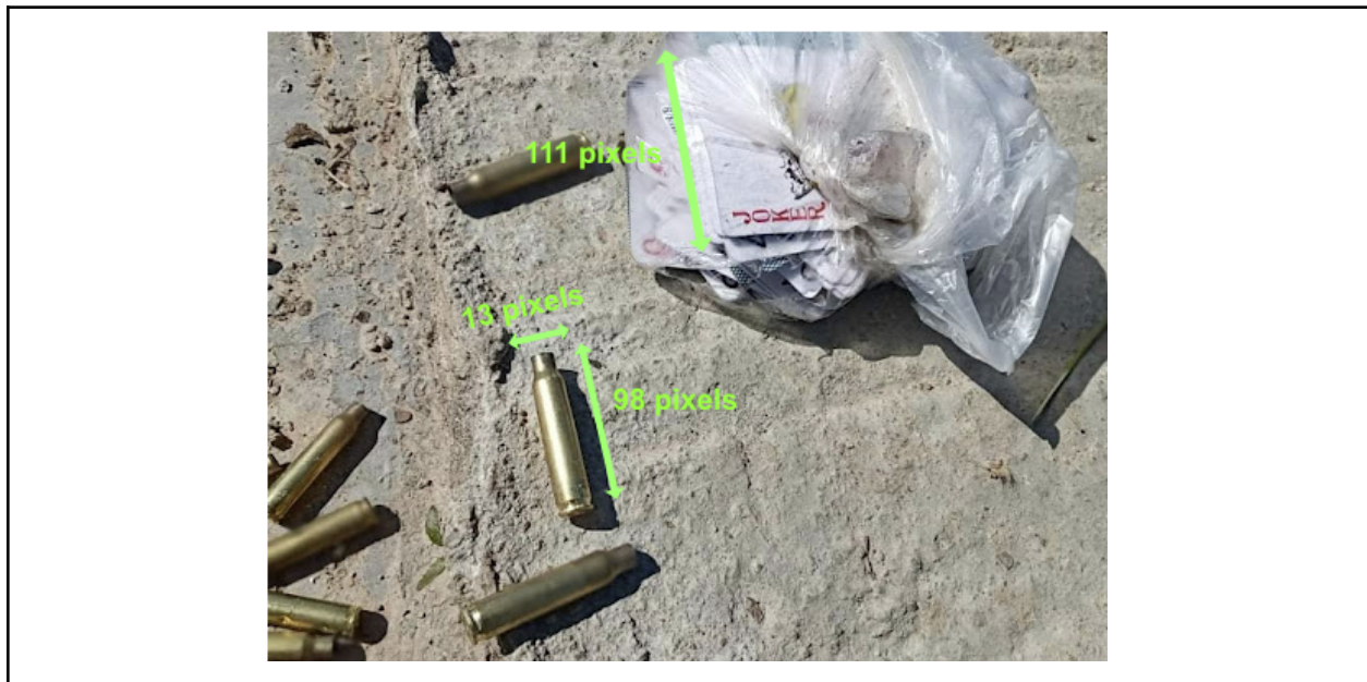
Figure 18: Pixel-ratio analysis indicates a rough specification of the cartridge size that exceeds that of 5.56 NATO rounds which would be typical of a modern SAC loadout. The calculation was based on standard playing card dimensions, where 111 pixels = 64mm; 1 pixel = 0.5766mm; therefore Cartridge length = 56.5mm and Cartridge shell width = 7.5mm. Minimum error is +/- minimum resolution, or +/- 0.5766mm though due to perspective, will be greater.
